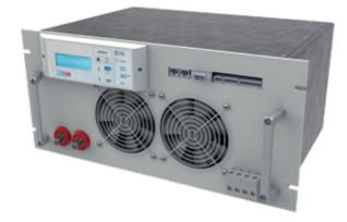
The ZB24DC300 series battery charger has been designed to charge batteries and supply DC loads of the rated voltage of 24 VDC – in co-operation with the battery. The charger may operate without the battery or with any type of battery. The charger incorporates the IGBT technology with primary switching, control is performed by the microcontroller, whose algorithm ensures:
