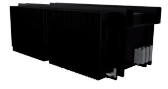
The PSM-44 auxiliary converter has been designed to convert 3000 VDC voltage used in the railway traction networks into 110 VDC and 24 VDC as well as 3×400 VAC and 220 VAC, used in the low voltage systems of EMUs (EN57). Auxiliary converter can be loaded with an unbalanced load of up to 6 kVA per line. In standstill conditions, (when the power supply with 3000 V is off) the converter may be powered from the 3×400 VAC industrial network.
