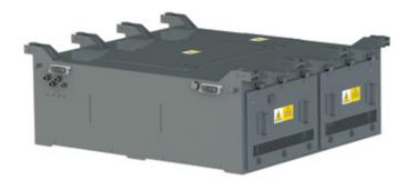
The auxiliary power unit PSM-230 (APU) were designed applying state of the art technologies: IGBT modules, Digital Signal Processors, modern magnetic materials, resin stabilization and others. The modern technological and circuitry solution provides excellent output parameters. The converter shares the input filter with the propulsion inverter that eliminates the fluctuations or transient inputs that may introduce noise into the equipment or from the APU to the catenary.
