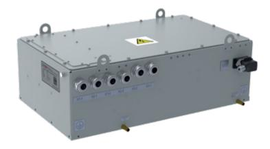
Fuel cell energy converter is intended for rolling stock applications. The converter, which uses full SiC technology, is designed for energy transfer from fuel cell to traction battery (charging). During operation fuel cell energy converter and traction battery are connected to propulsion system circuit. The converter transforms energy generated by the fuel cell into the energy used for charging the traction battery.
