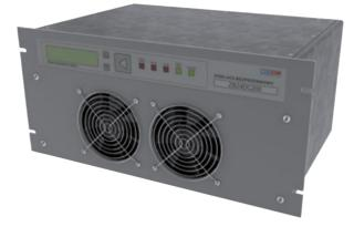
The ZB24DC200 series battery charger has been designed to charge batteries and supply DC loads of the rated voltage of 24 VDC – in co-operation with the battery. The charger may operate without the battery or with any type of battery. The charger incorporates the IGBT technology with primary switching, control is performed by the microcontroller, whose algorithm provides:
