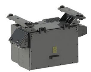
The device draws energy from a 3×400V 50Hz platform grid and converts it into the 24 V used in the LV carriage supply grid and for battery charging. The main features of the charger are: very good stability of the output voltage and temperature correction of the battery charging voltage. The device is fitted with a microprocessor control system which limits the output current in case of overload or short-circuits.
