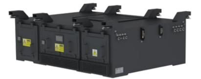
Auxiliary converter type PSM-195 has been designed to supply the circuitry of the railway vehicle with 3×380 V /60 Hz and 72 VDC. Input power supply for this converter is 3000 VDC. It is possible to supply the converter from a 3×380 V 60 Hz depot supply. The PSM-195 auxiliary converter is built-in in a tight metal housing made of aluminum. Some of these profiles are used for heat dissipation.
