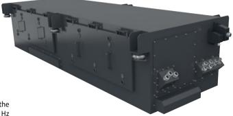
Auxiliary converter type PSM-160 has been designed to supply the circuitry of the railway vehicle with 3×380 V and 3×220 V, both 60 Hz and 72 VDC. Input power supply for this converter is 3000 VDC. It is possible to supply the converter from a 3×380 V 60 Hz depot supply. The PSM-160 auxiliary converter is built-in in a tight metal housing made of aluminum profiles and sheets. Some of these profiles are used for heat dissipation.
