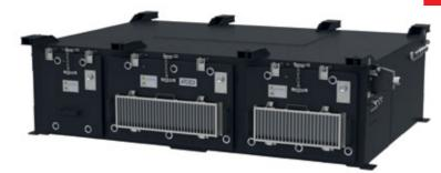
Auxiliary converter is a fully automated device designed for converting traction power supply voltage 750 VDC to 110 VDC, 3x415 VAC / 50 Hz and 230 VAC / 50 Hz of auxiliary circuits and batteries charging. The device uses technique of multiple conversion of energy. Constant voltage from the catenary line (750 VDC) is converted into alternating voltage and then rectified and transformed to obtain low DC voltage. The 110 V output voltage is adjusted to the char-
