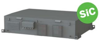
The power box and propulsion of the FT-50-600-Q-Combo tram consists of four FT-50-600 inverters and one PSM-50 SiC auxiliary converter. The FT-50-600 propulsion inverter is a device that transforms the input voltage from the pantograph into a three-phase alternating voltage of variable amplitude and frequency while maintaining a constant U/f ratio.
