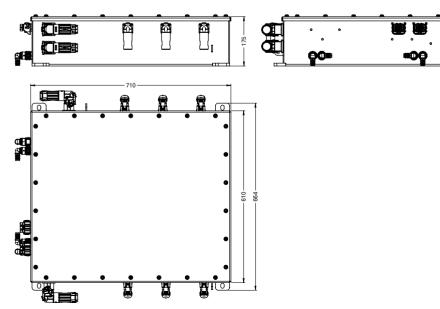
Modular Power Converters Set for Hydrogen Buses
