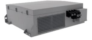
The application of independent inverters for powering of single motors guarantees high traction parameters, perfect performance at the slip point and no influence of non-uniform wear of wheels on the drive's performance. The FT-105-600D drive inverter is a modern module inverter incorporating the IGBT technology.
