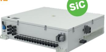
Propulsion inverter is designed to supply the motor or motors driving the wheels in an electric bus. Container of the inverter with HV switchgear and PSM auxiliary converter is designed for installation on the roof of the vehicle. Propulsion inverter is designed to be powered from the traction battery.
