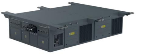
The traction container box is designed to power the traction motors driving the wheel axles in a metro vehicle. The device is designed for installation under the vehicle floor. Propulsion inverters are designed to be supplied by 750 VDC traction voltage. The drive units in the vehicle enable starting, driving with a given torque, coasting and braking the vehicle. They also enable starting, driving and braking with the set reverse travel direction.
