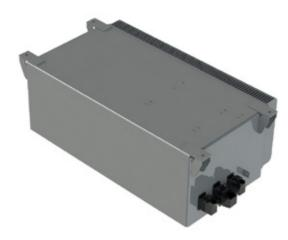
Static auxiliary converter PSM-8E is a device designated for the conversion of the input of the catenary's voltage of 600 VDC into auxiliary voltages of 100 VDC and  $2\times200 V 60 Hz$ .
