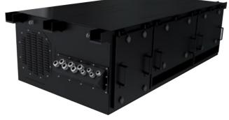
The PSM-132 auxiliary converter has been designed to convert DC voltage of the 750 VDC metro traction into  $3\times380$  VAC 60 Hz AC voltage, applied in the low voltage systems of metro, used to supply the auxiliary circuitry in the metro system, air conditioning and DC loads.
