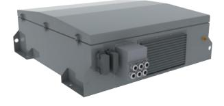
The PSM-60T auxiliary converter has been designed to convert DC voltage of the 600 VDC traction into 24 VDC voltage, as well as 3×400 VAC and 230 VAC voltage, needed to supply the auxiliary circuitry of the tram system, driver's air conditioning and car ventilation.
