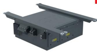
Auxiliary converter is a fully automated device designed for converting traction power supply voltage 750 VDC to 110 VDC and 3x400 VAC / 50 Hz of auxiliary circuits and batteries charging. The device uses technique of multiple conversion of energy.
